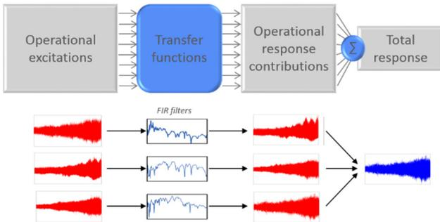
Figure 1: Independent relationships between multiple sources and receiver(s) in a simple system, allowing a direct measurement and analysis of each subcomponent independently
