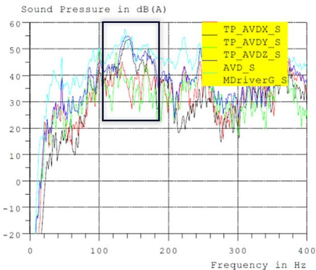
Figure 9: Front axle contributions compared to the global noise level (cyan curve)
