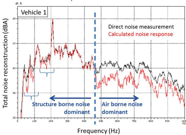
Figure 6: Comparison between measured noise and recalculated noise with OTPA method
