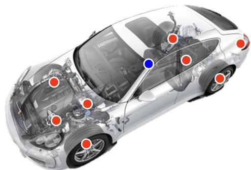
Figure 5: Example of OTPA instrumentation, with in blue a response channel, microphone at driver's ear, and in red the sources, 8 accelerometers for the hubs, engine, gear box and rear drive axle
