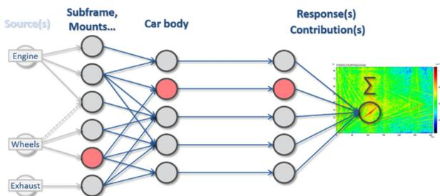
Figure 2: Complex relationships between multiple sources and receiver(s) in a real system such as a vehicle
