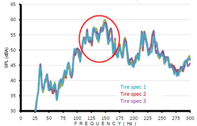
Figure 8: Noise measurement with different tire specifications
