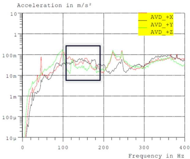
Figure 10: Acceleration measured at the front right hub (X : red curve, Y : black curve, Z : green curve)
