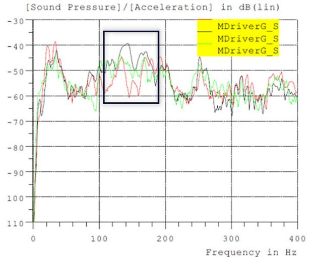
Figure 11: Transmissibilities for front right hub (X : red curve, Y : black curve, Z : green curve)
